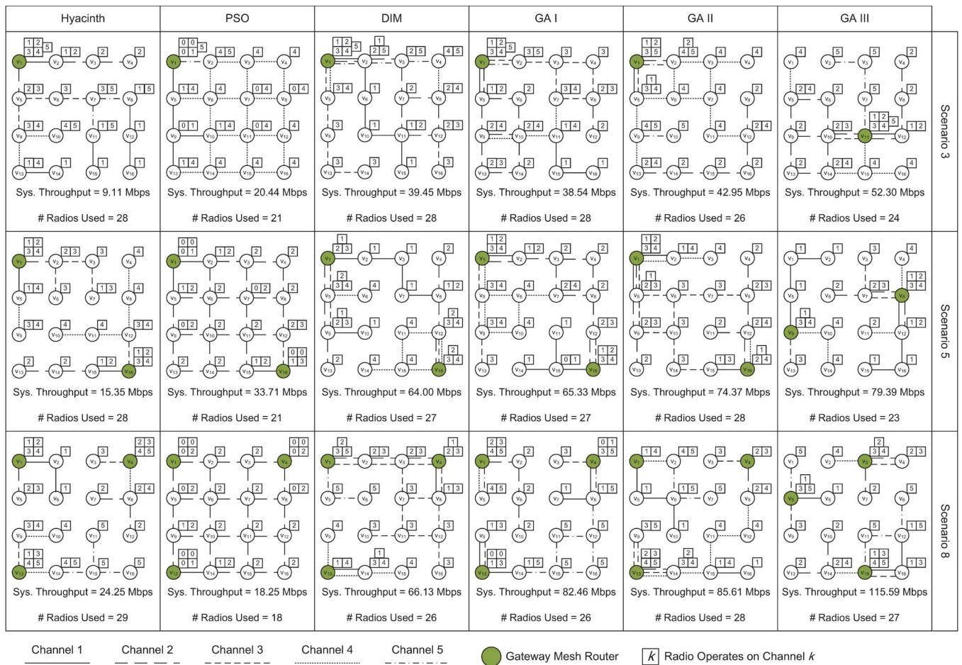
Fig. 11. Display of the resulting radio and channel configurations produced by the respective WMN optimization approaches when one gateway (scenario 3), two gateways (scenario 5), and three gateways (scenario 8) are available among mesh routers.
